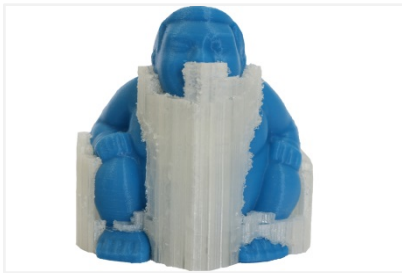
[Foto 6] Customized and water-soluble: The polymer Mowiflex from Kuraray is suitable for many applications ranging from injection molding to additive manufacturing. Demonstrably biodegradable in water, Mowiflex is the ideal carrier material in 3D printing and for the production of automatic dishwasher tablets.
